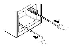
Grasp the drawer on each side and hook drawer supports (1) into rail tabs (2) located on both sides.
